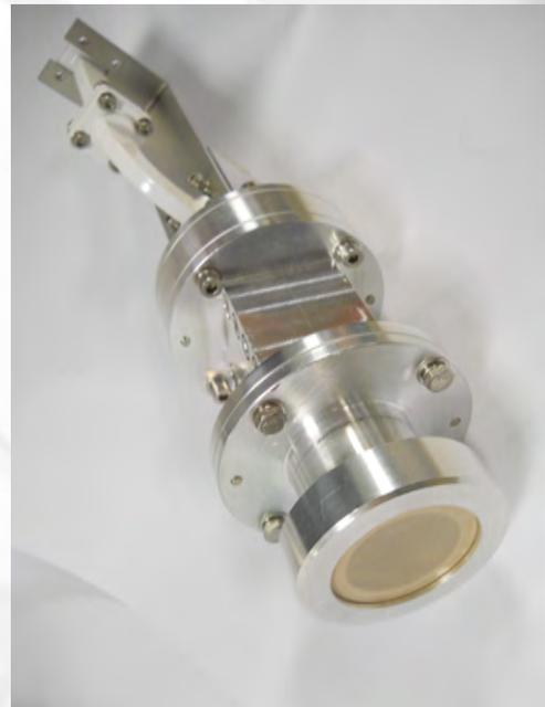
*Our Circular Ka band feed developed for use with Nilesat 201's Ka band transponders*
