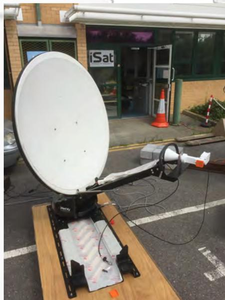
*Vehicle mount conversion from Ku to X-band for a customer in Canada*
